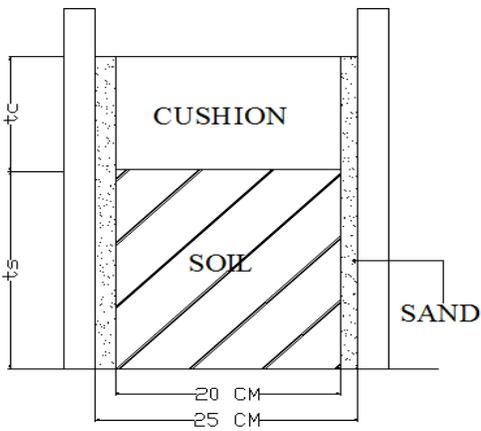
**Fig. 1 Schematic representation of sample preparation of soil-cushion layers for test**
