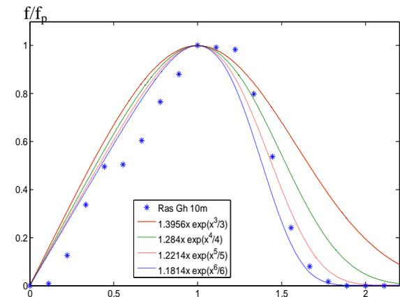
Fig. 4, Different alternatives of the model ( $n= 3,4,5$  and 6) compared to actual data of Ras Ghareb.
