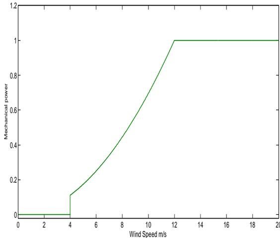
Fig. 7, The mechanical power versus the wind speed.
