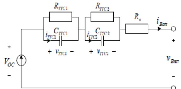
Figure 3. Battery equivalent circuit.
