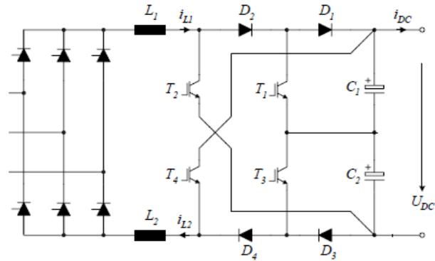
Figure 2, Bi-directional AC-DC converter with sinusoidal currents.
