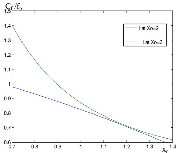
Fig. 8, I ( $C_f/f_p$ ) versus relative rated wind speed.
