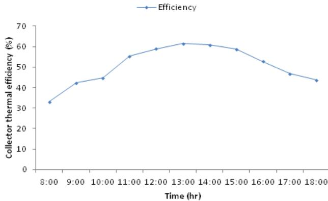
Figure 6: Variation of collector thermal efficiency with time
