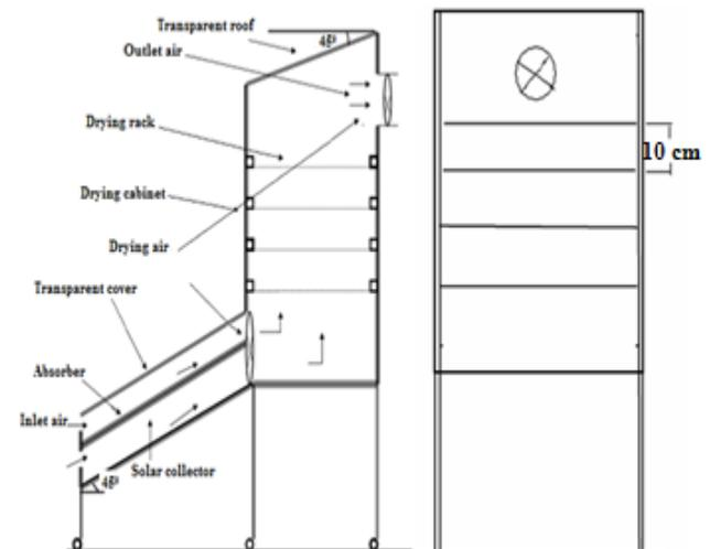
Figure 1: Features of the solar crop-drying system
