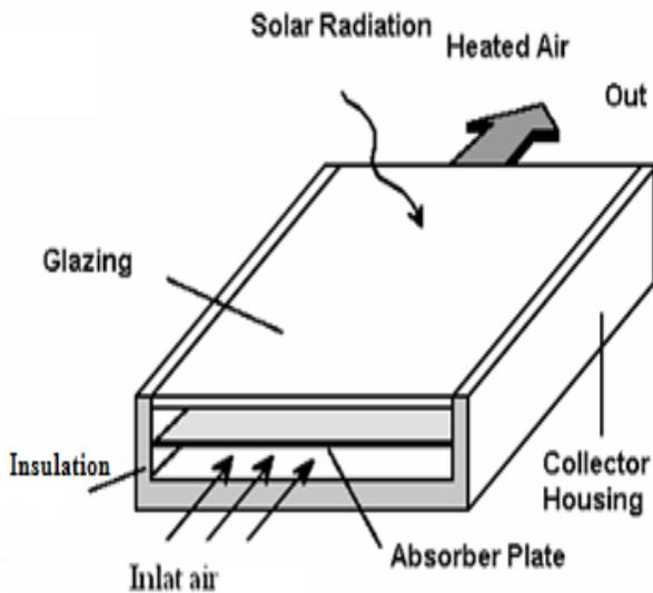
**Figure 2: Typical solar air collector**
