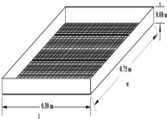
**Figure 3: The tray showing its dimensions**
