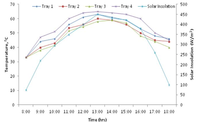
**Figure 4: Temperature variation of ambient air, drying air on each tray and insolation**
