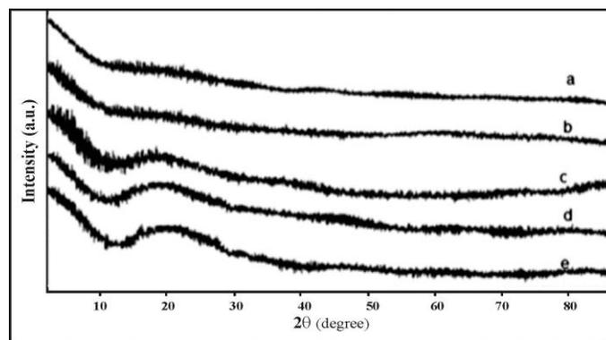
**Figure 1:-** XRD pattern for 1 drop RH6G dye doped (a) 0.5,(b)1,(c) 1.5,(d) 2,(e) 2.5 gm PVA+NH<sub>4</sub>SCN gel electrolytes.
