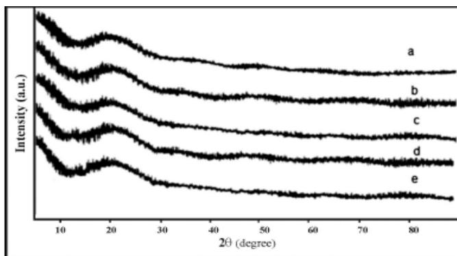
Figure 2:- XRD pattern for 2 drop RH6G dye doped (a) 0.5, (b) 1, (c) 1.5, (d) 2, (e) 2.5 gm PVA+ $\text{NH}_4\text{SCN}$  gel electrolytes.
