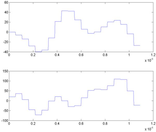
Figure5: Output of Transmit Filter in time domain
