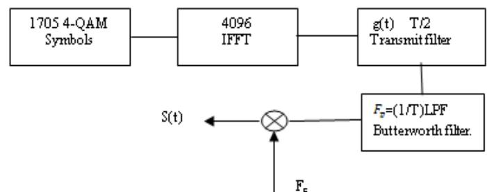
Figure 1. OFDM Transmission
