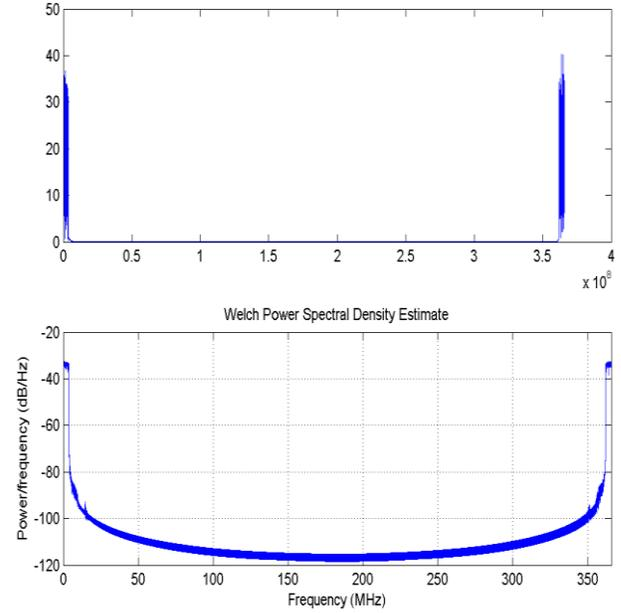
Figure9. Output of Butterworth filter in frequency domain
