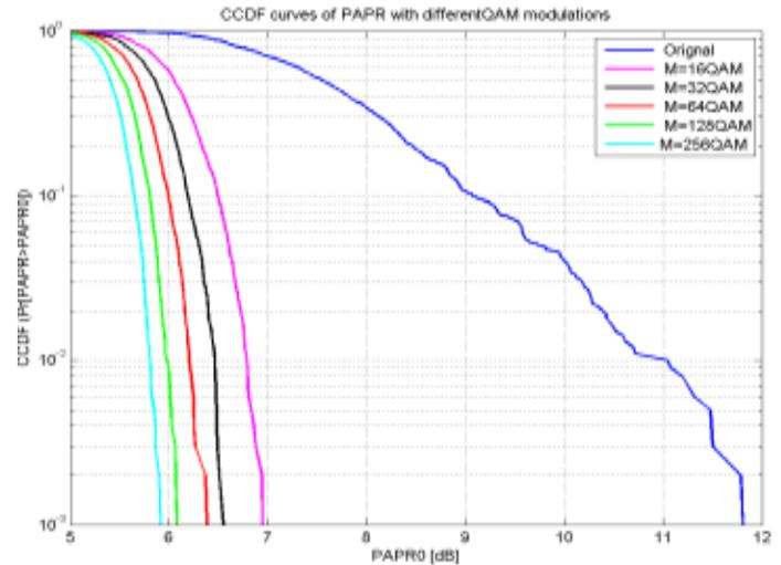
Figure 12. Plot for QAM constellations using conventional SLM
