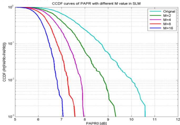
Figure 11. Plot for PSK constellations using conventional SLM
