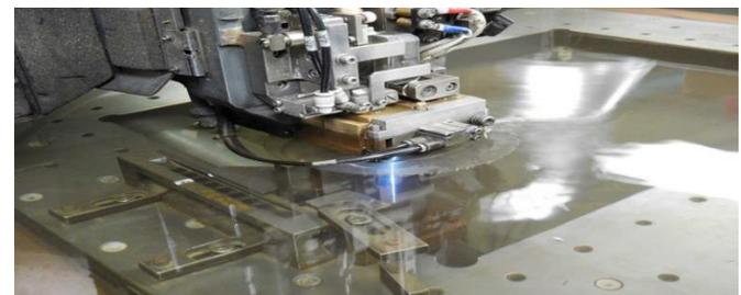
Fig.2: Experimental setup of a wire EDM [13].
