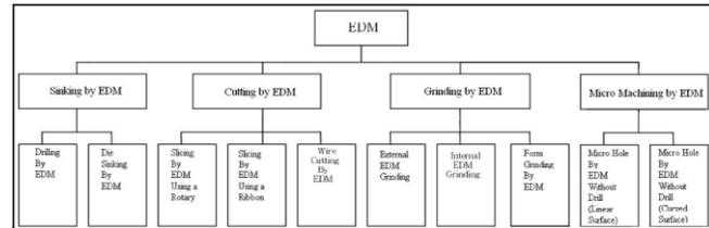
Fig. 1: Classification of the Spark Erosion Machining Processes [2].
