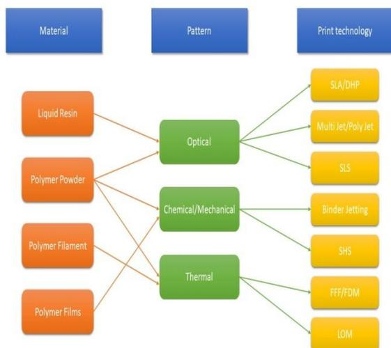
**Figure 1:** Polymer materials used with specific building methods in 3D printing.
