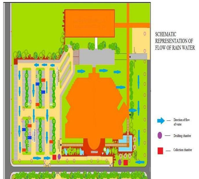
**Figure 4. Schematic Representation of Runoff to Recharge Structure”**
