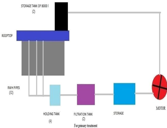
**“Figure 2. Schematic Representation of RWHP for Storage Purpose”**
