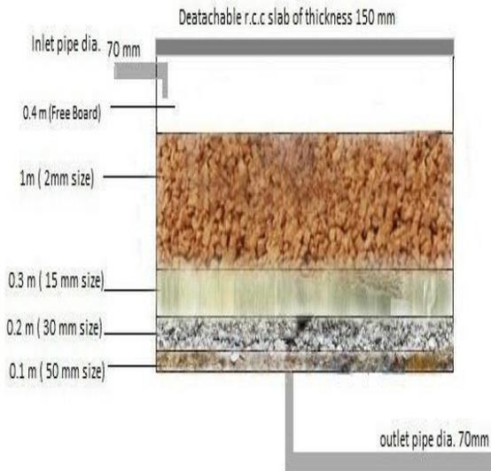
**”Figure 3. Slow Sand Filtration Tank for Primary Treatment”**
