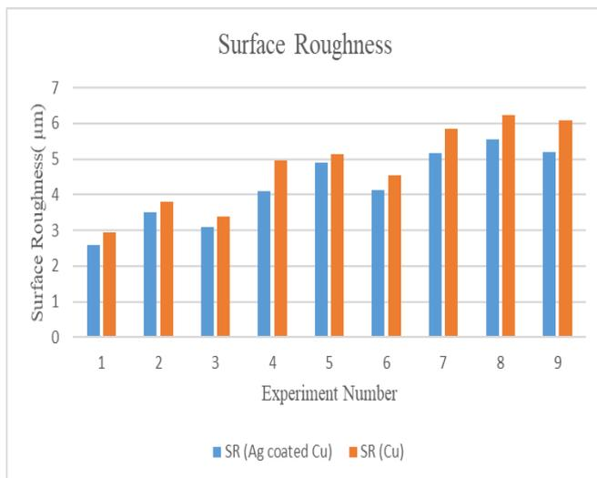
Figure 9: Comparison of SR between Ag Coated Cu and Cu electrodes.
