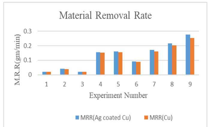
Figure 7: Comparison of MRR between Ag coated Cu and Cu electrodes.
