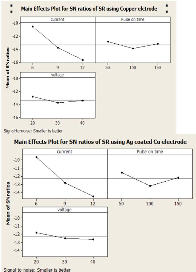
Figure 8: Main effect plot for surface roughness of AISID3 work piece using silver coated copper electrode and electrolytic copper electrode.
