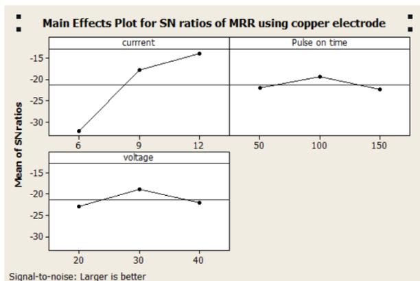
Figure 6: Main effect plots for material removal rate of AISID3 work piece using silver coated copper electrode and electrolytic copper electrode.
