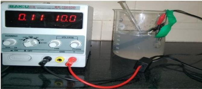
Figure 1 : Electroplating of silver on copper electrode
