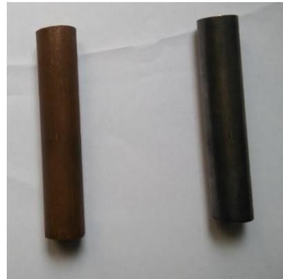
Figure 4: copper electrode and silver coated copper electrode used for EDM process
