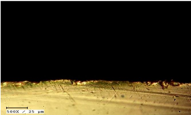
Figure 2: Microscopic view of silver coating using optical microscope
