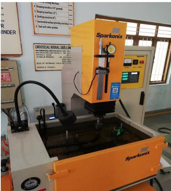
Figure 3: Electrical Discharge Machine used for the machining of AISI D3 steel
