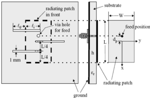
Fig 4: Design of compact microstrip antenna with meandering slots in the ground plane.
