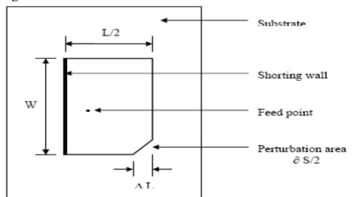
Fig 1: Configuration of microstrip antenna with shortedpinq4
