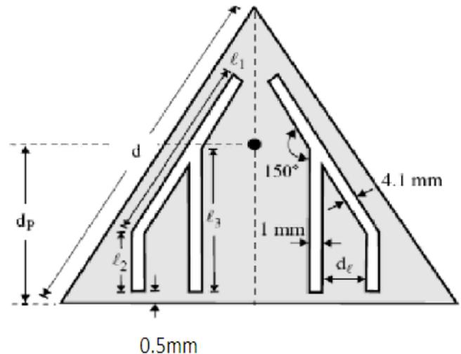
Fig 3: Slot loaded Triangular Microstrip Patch Antenna.
