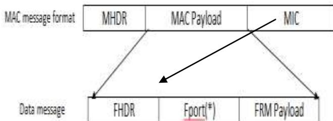
This is LoRaWAN Medium Access Control message format. The Fport(\*) field is present when the frame payload field contains data. The frame header (FHDR) field has a size of 7 bytes if it does not contain options, and up to 22 bytes when options are used (with an option size of up to 15 bytes). In this paper, we assume that options are not present in data messages.
