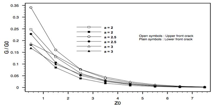
Fig.9: Propagation criterion  $G$  for both crack fronts at the same instant
