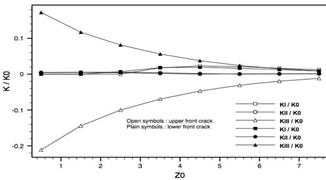
Fig.7: Stress intensity factors for both crack fronts at the same time for a radius loading disk  $a = 2.5$
