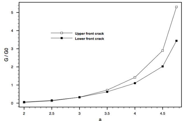
Fig.5: Propagation criterion according to the loading disk
