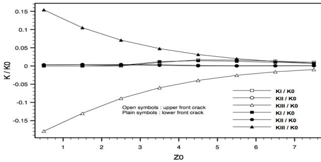
Fig.6: Stress intensity factors for both crack fronts at the same time for a radius loading disk  $a = 2$
