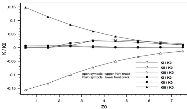
Fig.8: Stress intensity factors for both crack fronts at the same instant for a radius loading disk  $a = 3$
