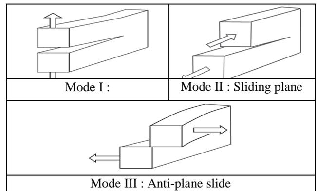
Fig. 1: Failure modes of a crack
