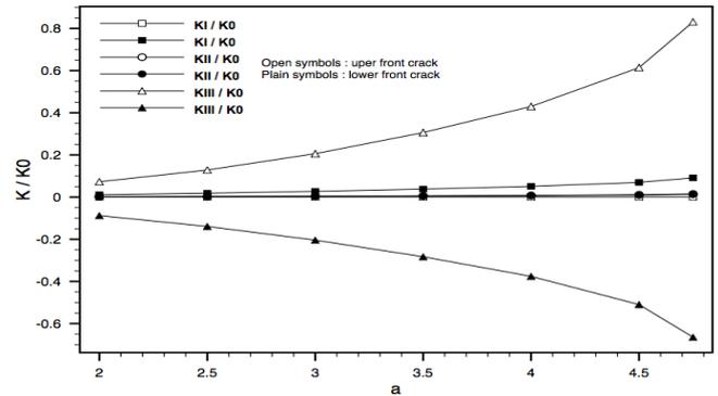
Fig.4: Stress intensity factors according to the loading disk
