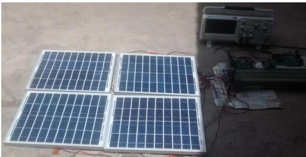
Fig. 3(b). Experimental setup with 2x2 mono-crystalline SPV array at NUI.
