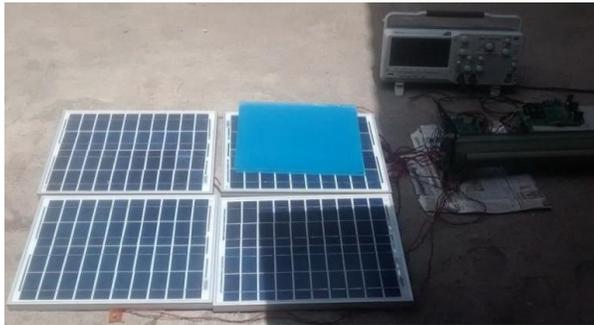
Fig. 3(a). Experimental setup with 2x2 mono-crystalline SPV array at uniform irradiation ( $740\text{W/m}^2$ )
