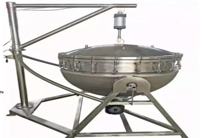
**Fig 2 Sealed vat pressure cooker**
